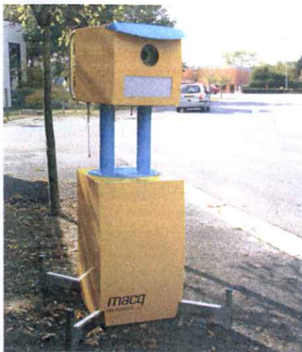
↑ Totem is an easy to set up mobile ANPR system
